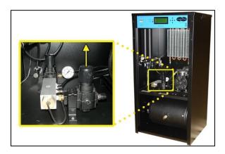
6.5.20.2 Turn knob untilOutlet Pressure(OUTLET) reading is at the desired setting.
