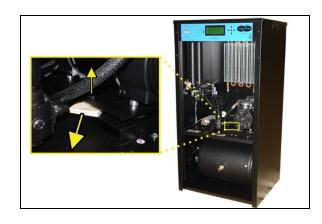
**6.5.6** Remove the ship-loose contents package.
